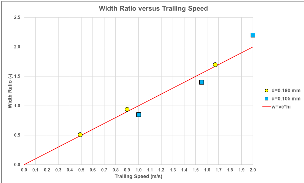
Figure 11-4. The effective width to penetration depth ratio, van Rhee (1986), (1987A) and (1987B) .
