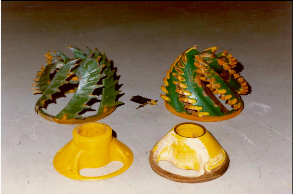
Figure 7-46: The crown cutter head (right), the short cone (left) and the long cone (right).
