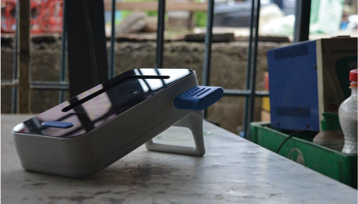
Figure 5-2: An optical instrument which allows anyone, not just experts, to diagnose malaria at a very early stage, using a simple pin-prick blood sample.
