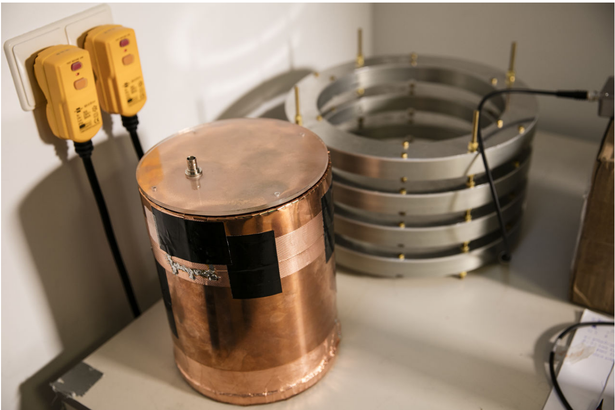
Figure 5-3: Elements of a frugal MRI.
