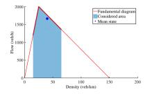
Figure 12.6: The construction of the average traffic state for two states on a triangular fundamental diagram.
