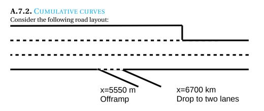
A three lane road has an offramp just downstream of 5500m, and a lane drop at approximately 6700m.
