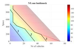
(b) XN-diagram and iso-t lines, with 3 trajectories. The colors indicate the time.
