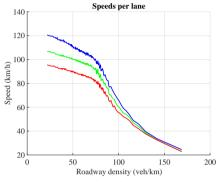
Speeds in the left lane are highest(1), so the graph with the highest fraction in the left lane is the flow (1), so the left figure is the flow (1). Similar reasoning (but the other way around) for right lane.
