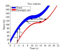
Figure 1.3: The microscopic variables explained based on two vehicles
