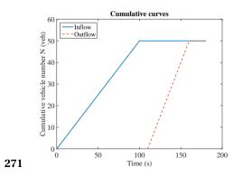
272 The delay is the area between the two lines (1).
