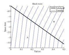
Figure 4.1: A shockwave where traffic speed changes from high to low.
