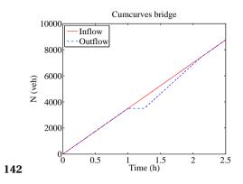
**143** In 15 minutes 3500/4=875 vehicles arrive, which are in the queue. After the bridge opens, the queue length reduces (3500 veh/h in 4500 veh/h out)
