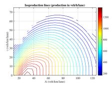
(b) Iso-production lines in the accumulation-inhomogeneity of density plane
