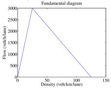
A piecewise linear speed-spacing diagram leads to a triangular fundamental diagram (0.5 – not asked in wording, but a wrong shape will get a reduction in points).
