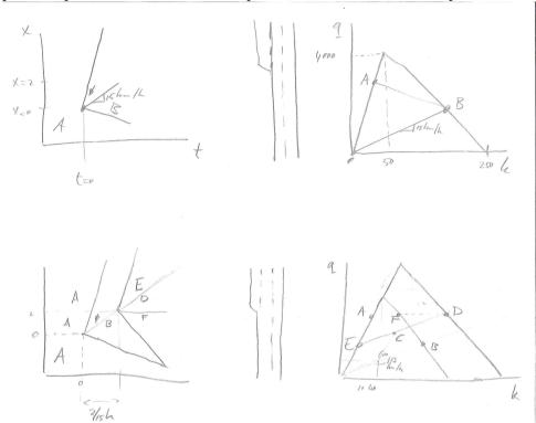
point F (1 point). Shock wave BF at the speed of the line BF in the FD (0.5 point).
