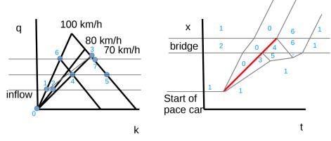
Solution 1: backward wave gets to the end of the bridge before the forward bridge reaches it
