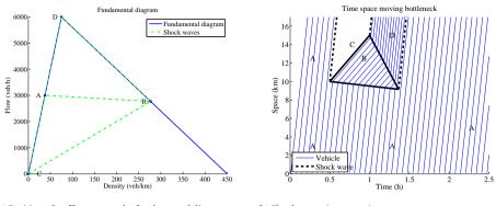
(a) Position of traffic states at the fundamental diagram (b) Shock waves in space-time
