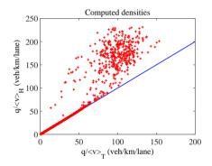
Figure 3.5: Densities computed using arithmic mean speeds or harmonic mean speeds; based on Knoop et al. (2007).
