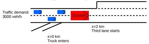
**Exercise 184.** *Sketch the traffic operations (both in space-time and in flow-density) for the time up to the moment the truck reaches the three lane section. (5 points)*
