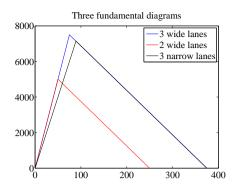
**149** The question relates to: where do the free flow line for 80 kms/h and the congested line cross. (0.5) The free flow line is: q=80k (0.5). The congested line is q=100\*25-25\*(k-25). (0.5) Setting q equal gives kc=29.8 veh/km/lane and q=2381 veh/h/l/lane. (0.5) For three lanes this gives 7129 veh/h. (0.5)
