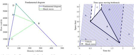
(a) Position of traffic states at the fundamental diagram (b) Shock w
