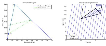
(a) Position of traffic states at the fundamental diagram
