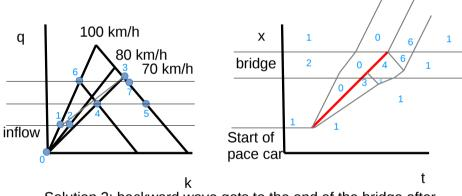
Solution 2: backward wave gets to the end of the bridge after the forward bridge reaches it
