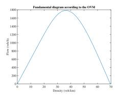
Figure 7.5: Fundamental diagram according to the OVM
