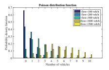
Figure 14.2: Example of the Poisson distribution for different flow values; the flow is indicated in veh/h, and these are the probabilities for arrivals in 15 seconds
