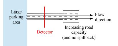
The above figure shows a simplified representation of the road layout. There is a detector at the red line, in the two-lane road stretch. Downstream of the detector the road widens and there are no further downstream bottlenecks.
