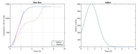
**261** The outflow curve increases when traffic starts to accumulate (1). The slope of the line is the outflow, given by the accumulation. If the accumulation increases to values over capacity, the outflow decreases, yielding a flatter outflow curve (1). Only when the inflow reduces to values under the low outflow, the accumulation decreases and the outflow increases again (1).
