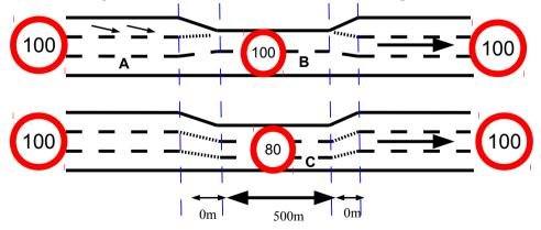
Throughout the question you may assume a triangular fundamental diagram for all road types. For the wide lanes, the critical density is 25 veh/km/lane and the jam density is 125 veh/km/lane. Assume the width of the lanes does not influence the congested branch.
