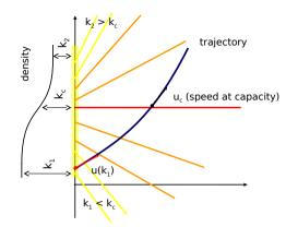
Figure 13.3: The kinematic waves (or characteristic curves) for an traffic situation where the upstream traffic state is overcritical and the downstream traffic state is undercritical
