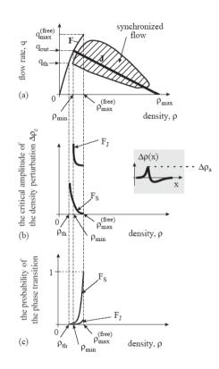
Figure 6.9: Transitions between the phases, figure from Kerner (2004)
