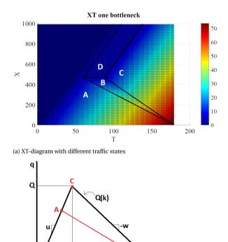
(b) Fundamental diagram with different traffic states
