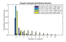
Figure 14.5: Example of the negative binomial function for the number of arrivals in an aggregation period
