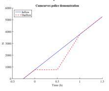
**206** The delay is given by the area between the two lines in the graph above (1). The max nr of vehicles in the queue ( $N_{\text{max}}$ ) is d \* qin. The time to solve is then  $t_{\text{solve}} = N_{\text{max}}/(C - q$ in) = d \* qin/(C - qin) (1). The area is  $1/2 * N_{\text{max}} * (d + t_{\text{solve}} (0.5))$ . Replacing the terms gives D = d \* qin \* (d + d \* qin/(C - qin). Further simplification (proof) leads to
