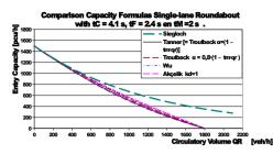
Figure 14.9: The inflow onto a road (or roundabout) as function of the main road (roundabout) traffic – figure from Fortuijn and Hoogendoorn (2015)
