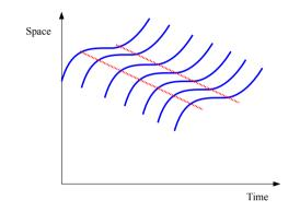
Figure 7.2: The average of the car-following behavior of drivers each with different parameters of the Newell model leads to a shock wave speed
