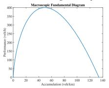
The performance on the vertical axis indicates the outflow out of the zone; the total road length in the network is 3.8 km. Assuming homogeneous and stationary traffic conditions, the following cumulative inflow and outflow curves are obtained:
