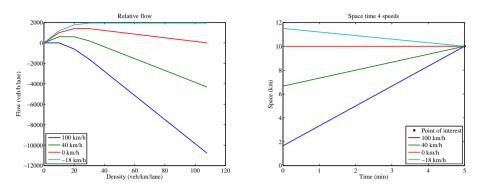
(a) The relative flows passing the different moving observers (b) The trajectories of the moving observers
