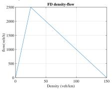
**291** We take the minimum of demand of cell 2 and supply of cell 3. Cell 2 is undercritical, and has a demand read from the fundamental diagram at k=20 veh/km (0.5), being
