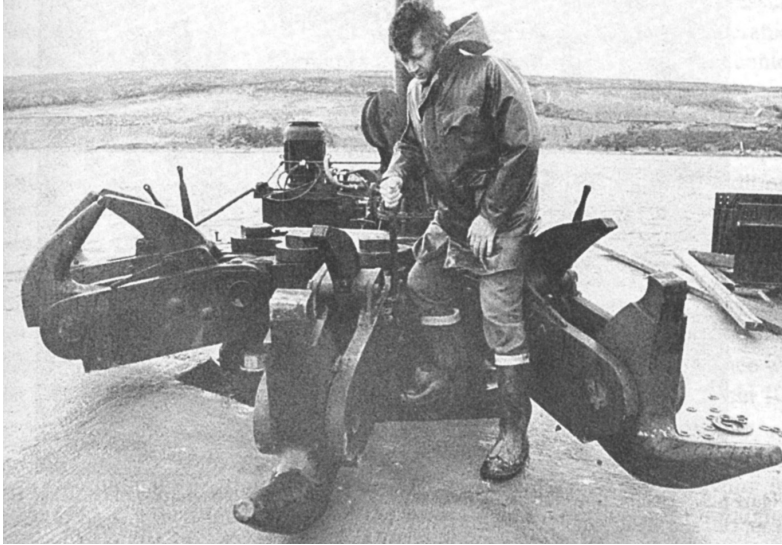
Figure 10.12 Multiple quick release mooring hook with a capacity of 150 tonnes per hook
