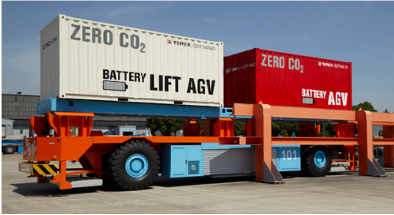
Figure 7.30: Lift Automated Guided Vehicle (Lift-AGV) (source: Terex® Gottwald)
