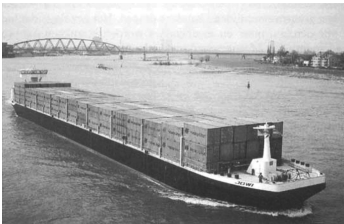
Figure 14.1 Container ship 'Jowi' has a capacity of 398 TEU
