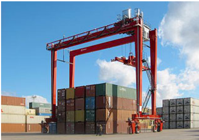
Figure 7.31: Rubber Tyred Gantry (RTG) (source: Kalmar)
