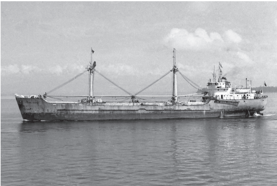
Figure 7.2 M.V. Clifford J. Rogers, the first ship specially designed as container vessel
