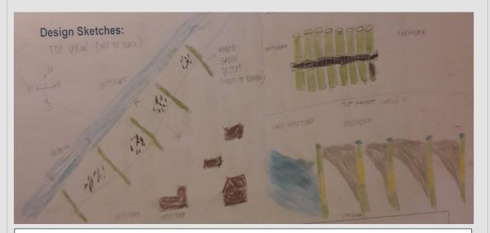
Design for cross-shore permeable groynes to be extended as sediment accretes nearer the coast. Photographs of the maquettes made to represent the design are included next.
