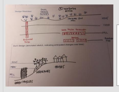
Design for a bamboo and green mussel breakwater located around mean sea level (MSL) with a geobag breakwater offshore of this and a mangrove planting area inshore of the shelter provided by the geobags and green mussels.
