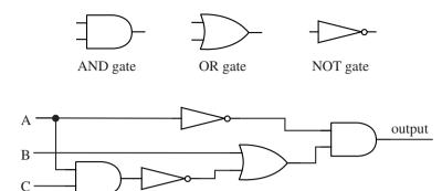
Figure 2.3: The standard symbols for the three basic logic gates, and a logic circuit that computes the value of the logical expression  $(\neg A) \land (B \lor \neg (A \land C))$ . The input wires to each logic gate are on the left, with the output wire on the right. Note that when wires cross each other in a diagram such as this, the wires don't actually intersect unless there is a black circle at the point where they cross.
