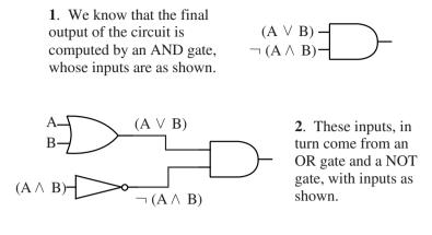
**3**. The circuit is completed by adding an AND gate to compute the input for the NOT gate, and and connecting the circuit inputs, A and B, to the apropriate gate inputs.
