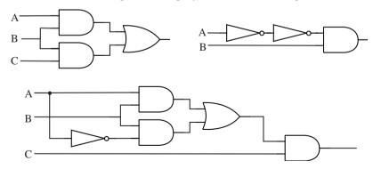
**8.** Design circuits to implement the input/output tables for addition, as given in Figure 2.8. Try to make your circuits as simple as possible. (The circuits that are
